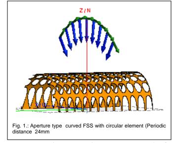
EM wave is incident on curved FSSs at various angles for diffrent stuctures with different periodicities. The transmission charecteristics of all the cases are noted down and are presented in fig.4, fig 5 and fig.6.
